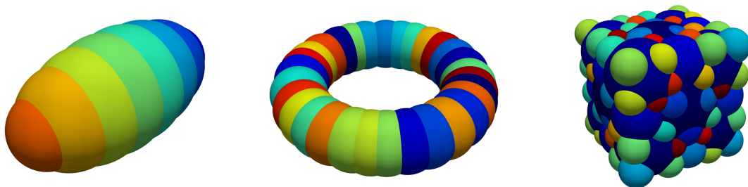
Figure 1: Multisphere representations of different geometries created by three clump generation method. From left to right, Favier, Ferellec-McDowell and Euclidean Distance Transform
